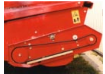
The simple, low-maintenance drive of the header auger and gathering unit.
